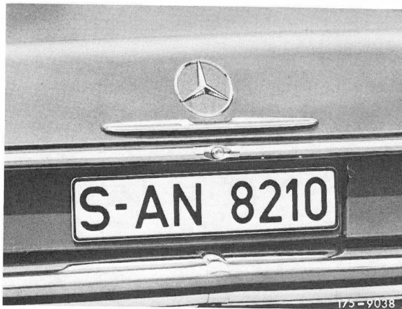
Fig. 50 Handle on trunk lid
